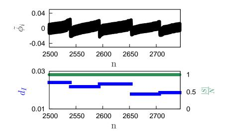
Figure 4.16: Example of a convergence process with real minimal transmission delay  $\tilde{\tau} = 0.01$ , whereas the theoretical bound is  $\tau_{\min} = 0.02$ . We show a close up when a certain level of synchrony is achieved. Due to the inaccurate delay bounds for  $H(\cdot)$  we see that  $d_I$  can increase. Note the small scale of fluctuations. Notation as in Figure 4.11  $(N = 100, \iota = 30, \text{ERG}).$
