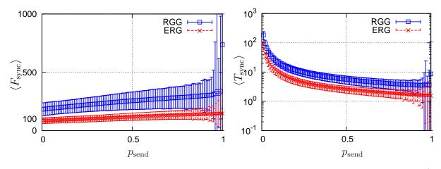
Figure 4.15: Synchronization performance depending on  $0 < p_{\text{send}} \leq 1$ , in terms of a) mean firing events and b) mean synchronization time. We only consider simulations runs that synchronize, which only affects the performance at  $p_{\text{send}} = 1$  (for all other parameters  $p_{\text{send}} < 1$ , all runs synchronized) (N = 100,  $\iota = 50$ ).
