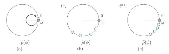
Figure 3.3: Alternative circular representation using  $\tilde{p}(\phi)$  from (3.5). The dark dot represents the phase position of the firing oscillator. Panel a) shows the smooth transition of the firing oscillator upon self-adjustment. Panel b) depicts an example for an ensemble of oscillators at a firing event at time  $t^n$ . Panel c) illustrates the phase positions right after the adjustments at time  $t^{n+}$  for a delay-free system.
