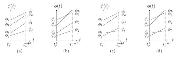
Figure 3.7: Examples of phase evolutions. Starting right after the phase adjustment at  $t_r^+ = t_o^n + \tau_{ij}$ , the phases evolve until the next firing event at  $t_o^{n+1}$ . Depending on the phase rates the leading and hindmost oscillator changes: a) no changes, b) change of leading oscillator, c) change of the hindmost oscillator, d) change of both hindmost and leading oscillator.
