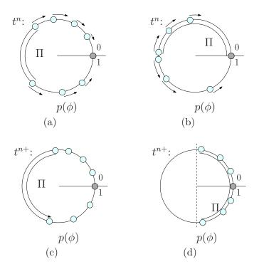
Figure 4.3: Demonstration of phase positions upon a firing event at time  $t^n$ . Setup as in Figure 4.2. At firing time all phases are spread over the whole interval [0, 1], see panel a) and b). In the first column, panel a) and c), the precision increases upon adjustments for low coupling strength. In the second column, panel b) and d), a large coupling strength gathers the oscillator phases within  $(\frac{3}{4}, 1] \cup [0, \frac{1}{4}]$ .
