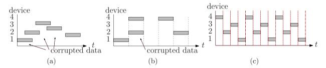
Figure 2.1: Three examples of communication protocols (dotted lines indicate slots, dashed frames). Panel a) depicts the ALOHA protocol, devices transmit data whenever needed. Panel b) depicts the slotted ALOHA protocol. At the beginning of very slot, devices transmit data if needed. Panel c) depicts the TDMA protocol. Devices are assigned to time slots for communication.
