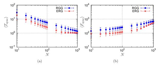
Figure 4.12: Mean synchronization time depending on the network size. Panel a) shows decreasing synchronization time with increasing network size  $(\iota = \frac{N}{2})$ . Panel b) shows moderate increase of the mean number of total firing events  $\langle F_{\text{sync}} \rangle$  to reach synchronization with increasing network size  $(\iota = \frac{N}{2})$ .
