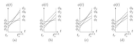
Figure 3.8: Examples of phase evolutions when both hindmost and leading oscillator change. Starting right after the phase adjustment at  $t_r^+ = t_o^n + \tau_{ij}$ , the phases evolve until the next firing event at  $t_o^{n+1}$ . Depending on the phase rates the leading and hindmost oscillator changes. Panel a) - d) show different situations how both leading and hindmost oscillators can change due different phase rates.
