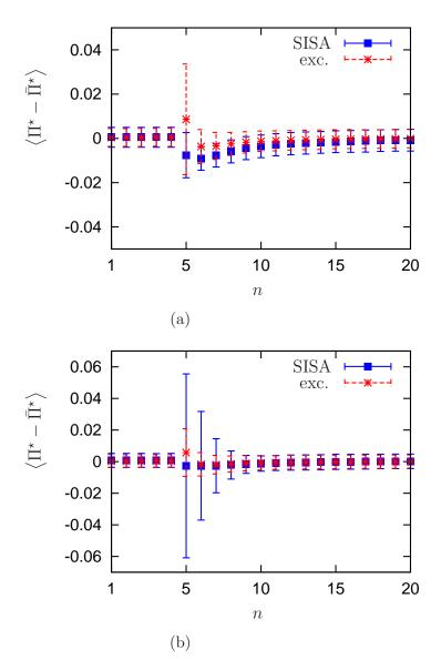
Figure 3.10: Precision disturbance from the synchronized state as a reaction to a false fire at cycle 5. Panel a) shows the performance for coupling strength  $\alpha_{\text{excitatory}} = 0.99$  and  $\alpha_{\text{inhibitory}} = -0.99$ , panel b) for coupling strength  $\alpha_{\text{excitatory}} = 0.5$  and  $\alpha_{\text{inhibitory}} = -0.5$ .
