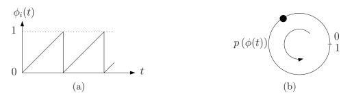
Figure 2.2: Two representations of the phase evolution. The phase increases linearly until it is reset. Panel a) shows the periodic behavior and the phase jump upon reaching the threshold 1. Panel b) show the a smooth transition of the phase upon reaching the threshold, due to the circular representation via  $p(\phi)$  as introduced in (2.13).
