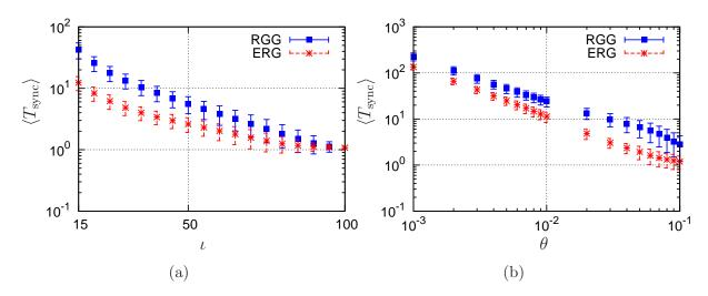
Figure 4.13: Dependence of mean synchronization time. Panel a) shows a decreasing mean synchronization time with increasing average node degree  $\iota$  (N = 100). Panel b) shows an increase of  $\langle T_{\rm sync} \rangle$  with decreasing synchronization bound (N = 100,  $\iota = 30$ ).
