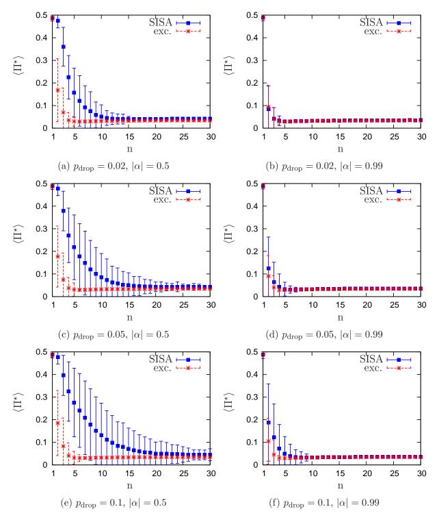
Figure 3.13: Failure of pulse detection. We show the mean normalized precision, starting from random initial conditions. Wit a probability  $p_{\rm drop}$  a received fire is dropped by an oscillator. We see that both algorithms can cope with the faulty behavior. The lower  $p_{\rm drop}$ , and the higher the coupling strength, the better the performance. With  $|\alpha| = 0.5$  the convergence of excitatory coupling is significantly faster, with  $|\alpha| = 0.99$  this difference vanishes.
