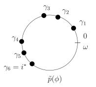
Figure 3.4: The index permutation of the oscillators. According to the alternative circular representation  $\tilde{p}(\phi)$  from (3.5) the oscillators are denoted in ascending order. The oscillator at the largest arc is denoted by  $i^*$ , as in (3.6).
