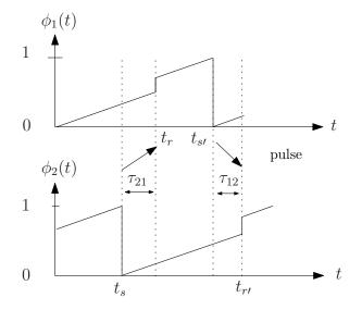
Figure 2.6: An example of the effect of individual random delays. We plot the phase evolution of two oscillators. At time  $t_s$  oscillator 2 emits a signal which is received by oscillator 1 with a delay  $\tau_{21}$ . The adjustment of oscillator *i* hence happens at  $t_s + \tau_{21}$ . Also, the pulse emitted by oscillator 1 at  $t_{s'}$  is delayed by  $\tau_{12}$  and received at  $t_{r'}$ . These delayed adjustments can add stochasticity to the system dynamics.
