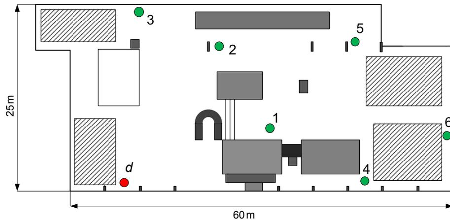
Figure 5.3: Factory layout and deployed sensor network.
