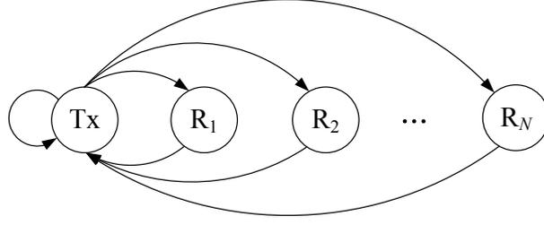
Figure 4.3: Protocol states and transitions for cooperative ARQ with proactive relay selection.
