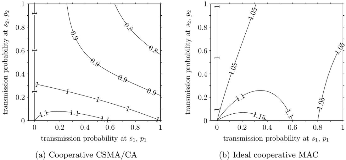
Figure 3.9: Ratio of overall network throughput with and without cooperation,  $\eta_{co}/\eta$ , as a function of transmission loads  $p_1$  and  $p_2$  in the non-symmetrical network scenario;  $\varepsilon_1 = \varepsilon_2 = 0.2, \varepsilon_{R_1} = 0$ .
