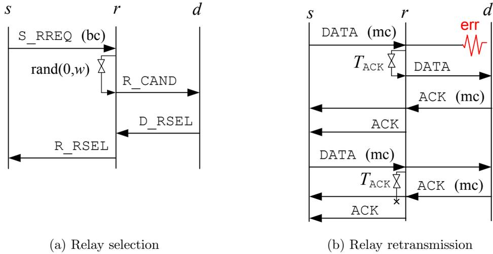
Figure 5.1: Message flow for periodic and adaptive relay selection (a) and relay operation after it is selected (b). Here and later in the text,  $bc$  and  $mc$  stand for a broadcast and a multicast transmission, respectively.
