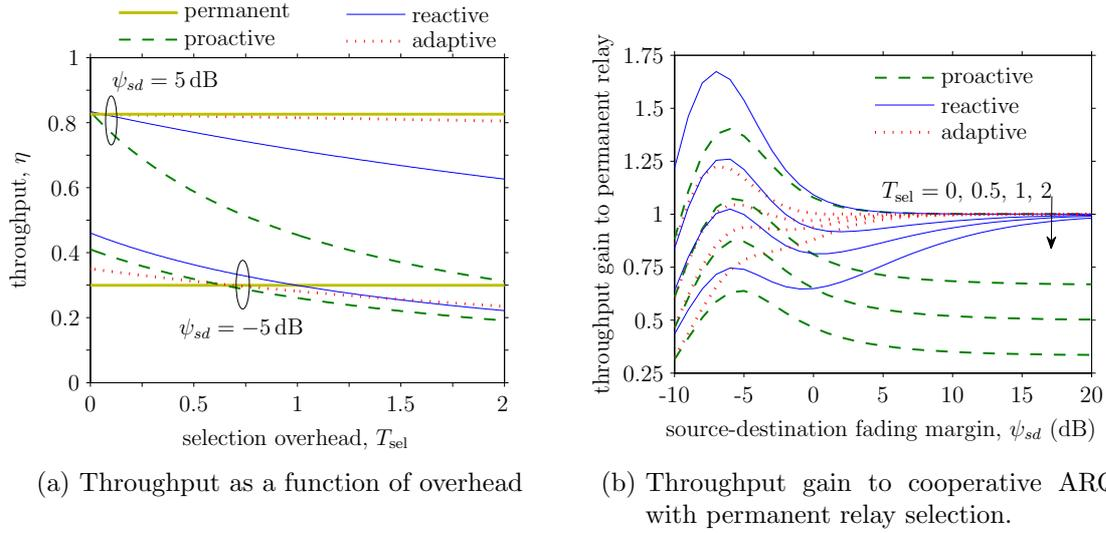
Figure 4.10: Impact of selection overhead on throughput;  $N = 5$ ,  $f_D T = 0.1$ .
