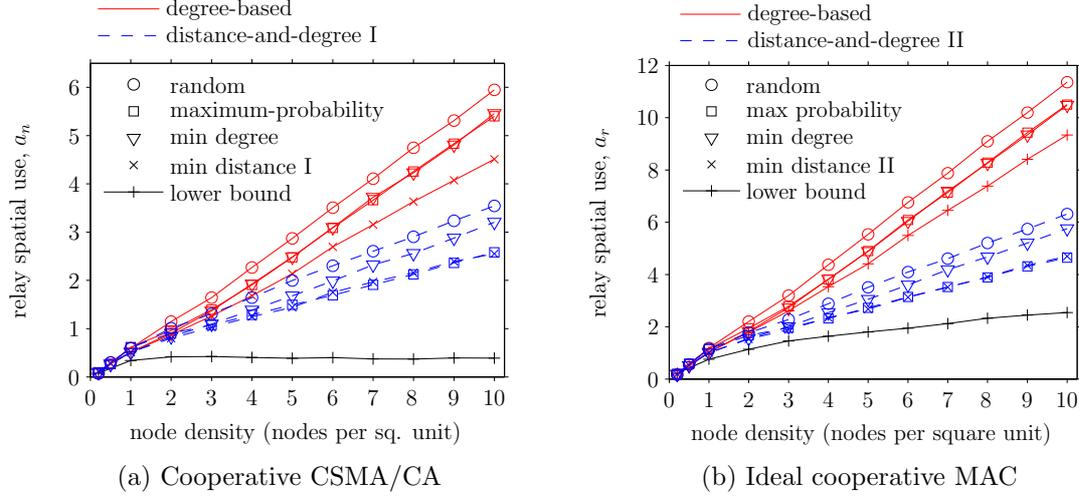
Figure 3.11: Expected relay spatial use  $a_r$  versus node density in the network for different combinations of utility and selection functions; contention window size  $w = 5$ .
