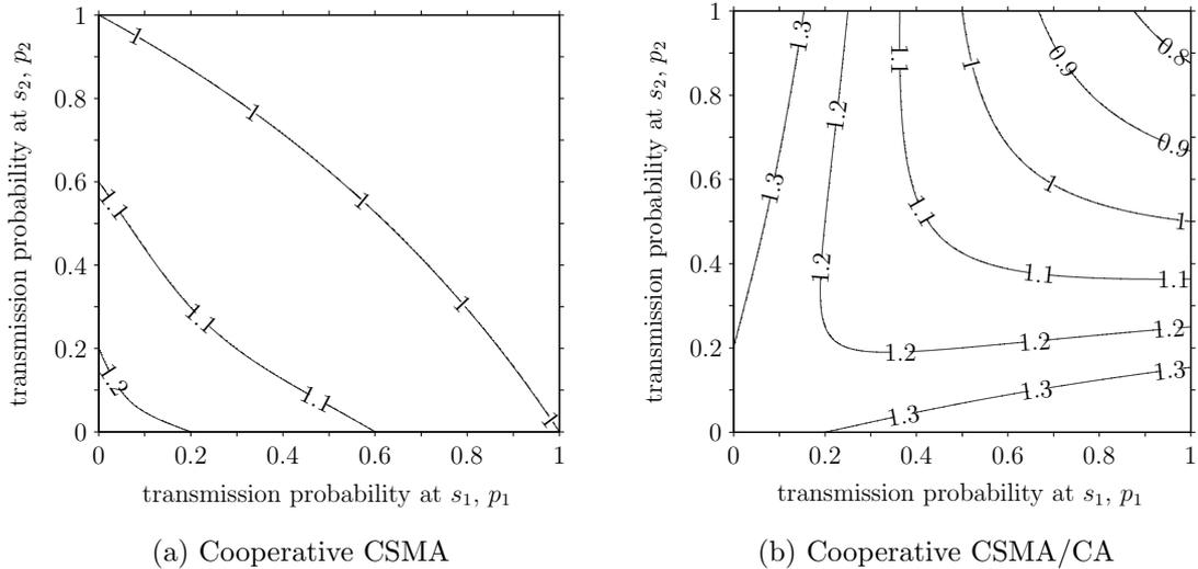
Figure 3.5: Ratio of overall network throughput with cooperation to that without cooperation,  $\eta_{co}/\eta$ , as a function of transmission loads  $p_1$  and  $p_2$  in the symmetrical network scenario;  $\varepsilon_1 = \varepsilon_2 = 0.2$ ,  $p_{R_1} = p_{R_2} = 0$ .
