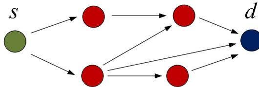
Figure 2.5: An example of routing with cooperative relaying.
