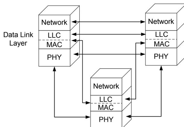
Figure 2.2: A protocol stack incorporating cooperative relaying.
