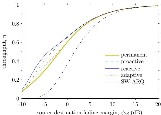
Figure 4.8: Throughput  $\eta$  as a function of source-destination fading margin  $\psi_{sd}$ . Number of potential relays  $N = 5$ , channel time correlation  $f_D T = 0.1$ , selection overhead  $\text{sel} = 0$ .
