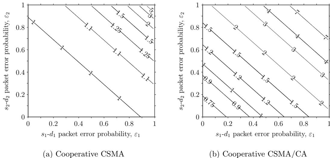
Figure 3.6: Ratio of overall network throughput with and without cooperation,  $\eta_{co}/\eta$ , as a function of packet error rates  $\varepsilon_1$  and  $\varepsilon_2$  in the symmetrical network scenario;  $p_1 = p_2 = 0.75$ ,  $p_{R_1} = p_{R_2} = 0$ .
