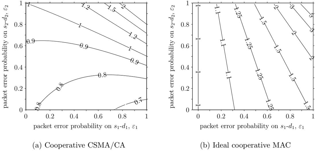
Figure 3.8: Ratio of overall network throughput with and without cooperation,  $\eta_{co}/\eta$ , as a function of packet error rates  $\varepsilon_1$  and  $\varepsilon_2$  in the non-symmetrical network scenario;  $p_{R_1} = 0, p_1 = p_2 = 0.75$ .
